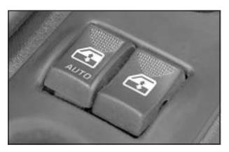
Both doors have power window switches located on the armrest. Press the front of the switch to raise the window. Press the back of the switch to lower it. The switches on the driver's door armrest control each of the windows when the ignition is in ON, ACC, or when Retained Accessory Power (RAP) is active. See Retained Accessory Power (RAP) on page 2-17.
